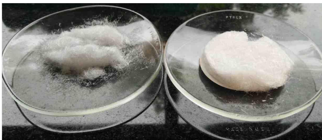
Figure 7: Crystal Produced at 65 °C (left) vs. at 105 °C (right)
