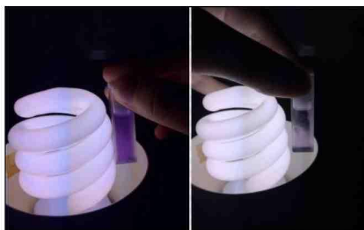
Figure 5 - Dye fatigue, the same sample before (left) and after (right) following repeated exposure to UV
